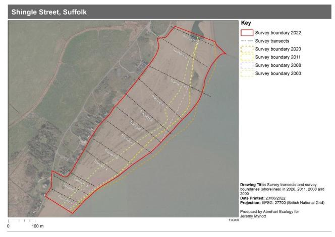
Figure 2- Aerial image showing increases in shingle accretion from 2000 - 2022 at Shingle Street.
